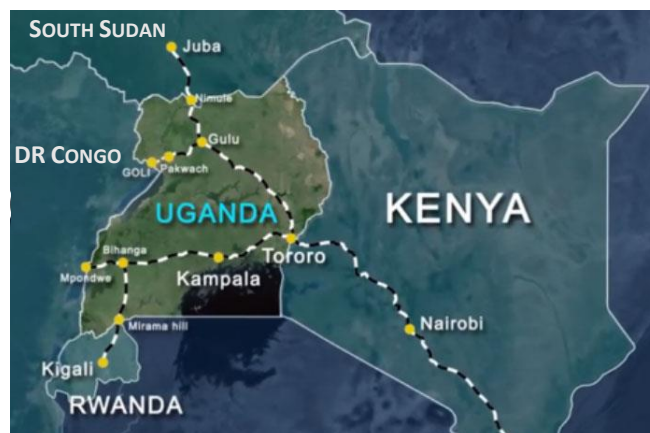
Figure 4: In Uganda, the SGR network will comprise four routes of total route length 1,724 km (subject to design modifications and sidings or branch lines). Source: Uganda SG Railway.
